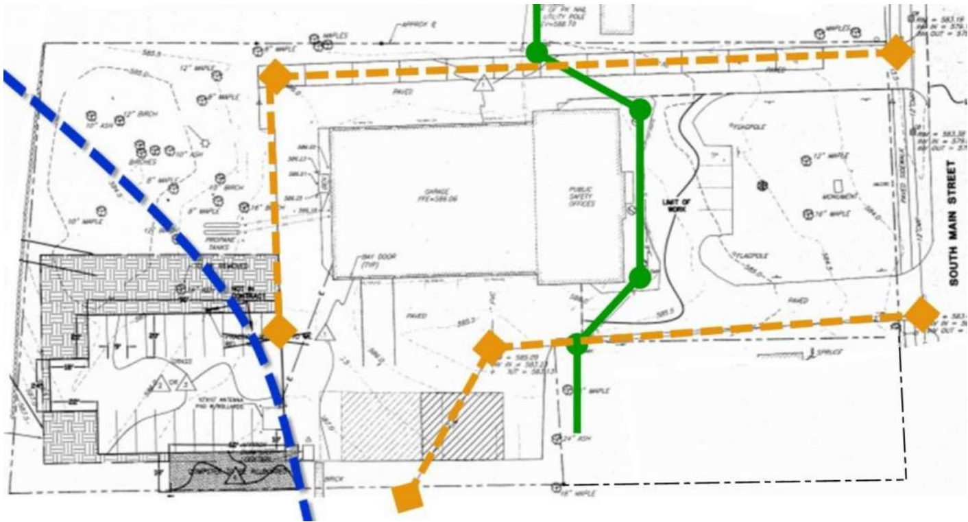
Existing Conditions Site Plan (Green = Sewer Line, Orange = Drain Lines, Blue = Drainage High Point)
