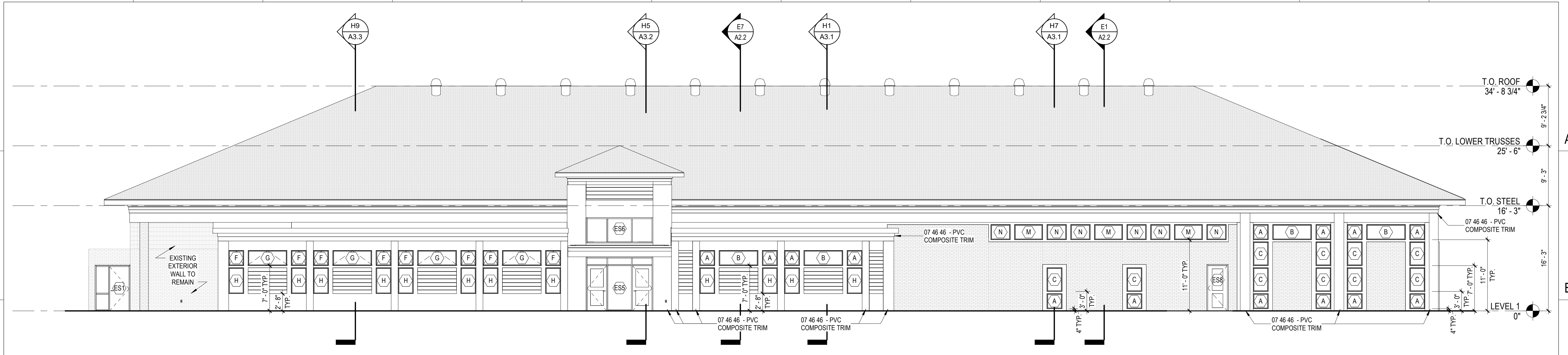
C1 EXTERIOR ELEVATION - SOUTH A2.1 1/8" = 1'-0"
